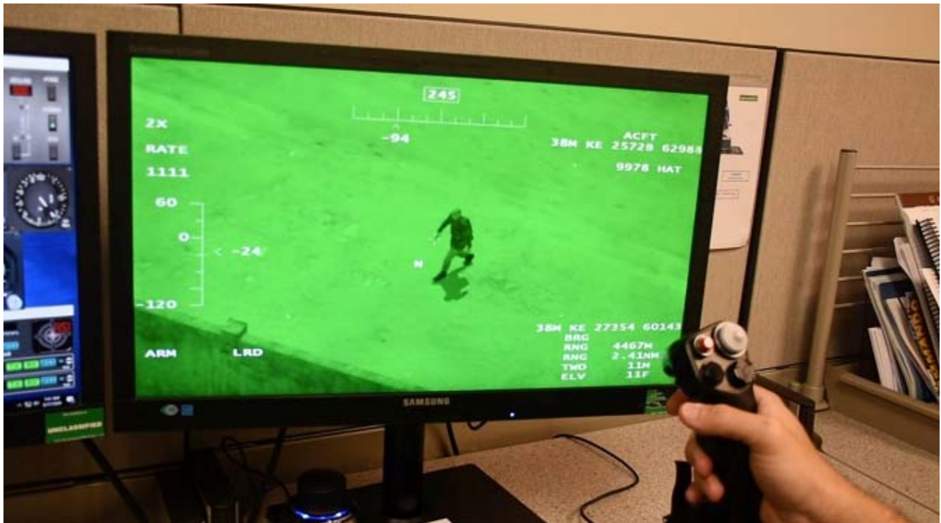
The SO laboratory replicates the entire mission profile scenario, including EO/IR sensor operations, tactical navigation, and countermeasure employment. Photograph provided by Major Sean Leuschen.
