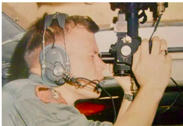
A navigator taking a celestial fix using the D-1 Kollsman periscopic-bubble sextant in the C-124C. Photo provided by Ron Barrett.
