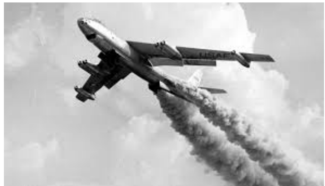
B-47 Rocket-Assisted Takeoff (RATO) bottle launch. Note: The navigator’s ejection seat shot downward. Photo from Wikimedia Commons.
